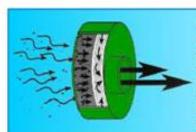
U.S.SAFETY's cartridges are uniquely designed with a space plenum between the filtering material and the inhalation port. Inhaled air is evenly distributed across the filter which lowers breathing resistance and extends cartridge life.
