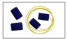
Manufactured from dependable PVC foam, these Therma-Soft 30™ earplugs are much softer than the competition. Slower "recovery time" allows for deeper insertion and a more secure fit. Improved foam responds to body heat by getting softer with use. Plugs are bright blue and available with or without cord. Packaged in poly bags 200 pair per dispenser uncorded, 100 pair corded. 10 dispensers per case. NRR=30 dB, CSA Class AL
